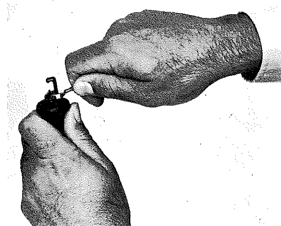
Figure 3. Cap Removal Tool. Use the cap removal tool, part number 001878, to loosen caps after centrifugation.
