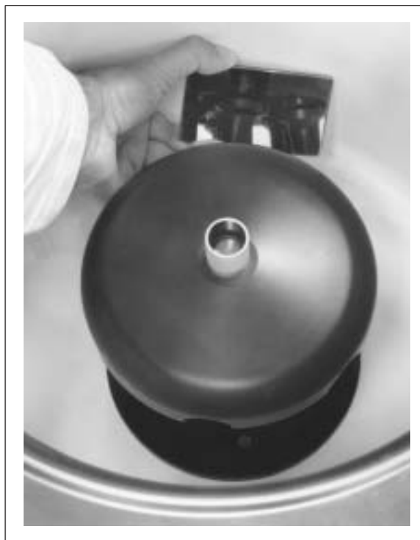
Figure 5-2. Checking Hook-on Bucket Positions After the Rotor is Installed. Note the partially unhooked bucket on the right.
